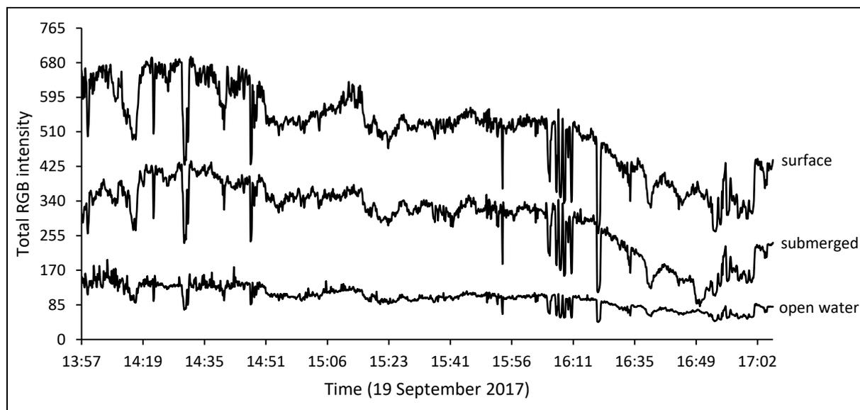
**Figure 1. Total RGB intensity measured for the white surface reference target (surface), the submerged target, and the open water area adjacent to the surface target.**
