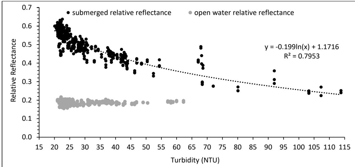
**Figure 2. Scatter plot of relative submerged reflectance (white reference submerged target reflectance/white reference surface target reflectance) and open water reflectance (open water reflectance/white reference surface target reflectance) and corresponding turbidity.**
