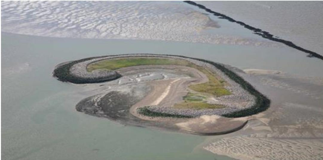
Globally for all the different works, the design allowed use inside the project of some 26 Million m<sup>3</sup> out of the total 45 Million m<sup>3</sup> to be dredged for new channel and basin.
