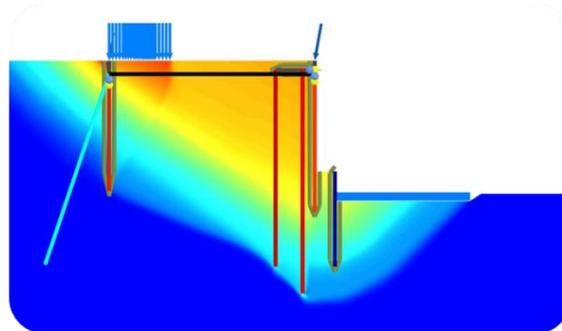
Figure 3: Typical cross-section of the refurbished quay wall (copyright: VCGP)
