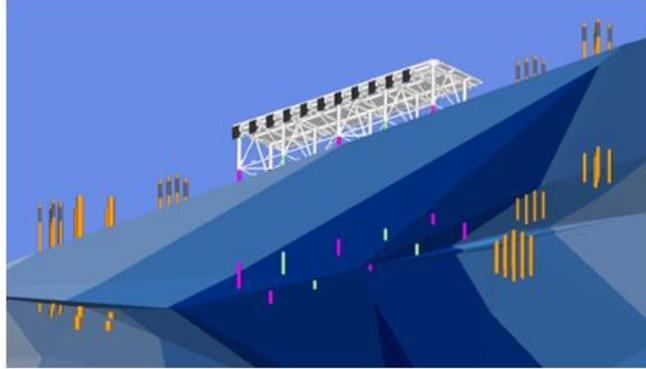
Figure 1: 3D Model of the seabed bearing substrate/layer
