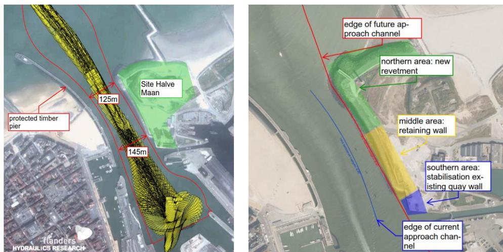
Figure 1: navigation simulation with widened approach channel and definition of project zones
