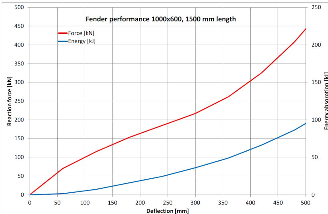
**Figure 7: Energy-Displacement diagram 1000 x 600 fender, 1500 mm length, according to supplier catalogue**
