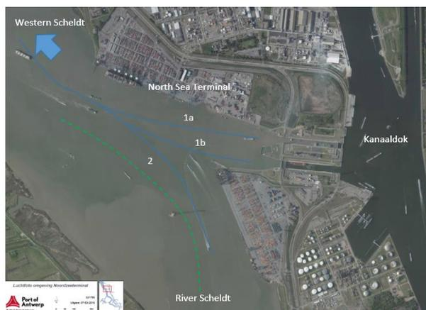
**Figure 1 : Port Of Antwerp ; Location North Sea Terminal; Three examples of passing trajectories (blue) and edge of navigational channel (green dash).
