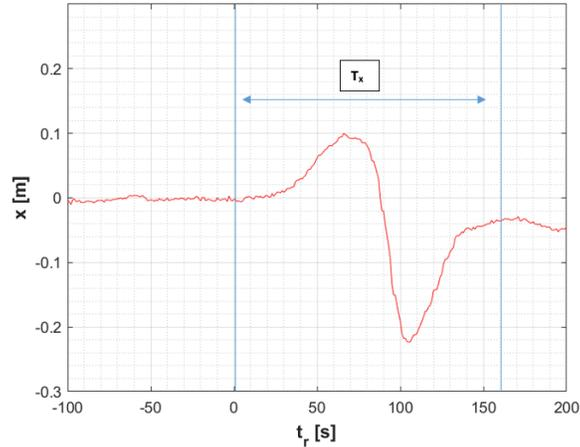
**Figure 2 : GPS registration longitudinal motion of moored Neo-Panamax container vessel with passing oil tanker.**
