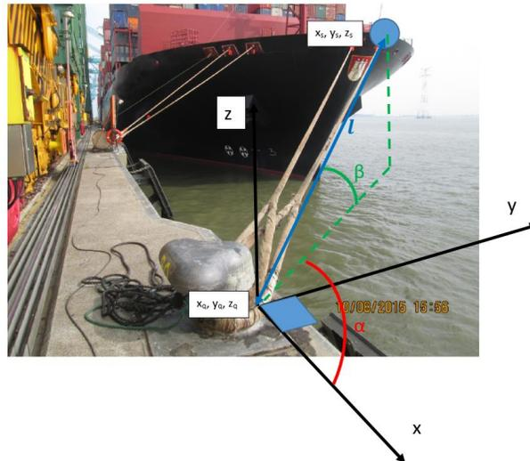
**Figure 3 : Definition line angles  $\alpha$  and  $\beta$  and the length of the line section between bollard and fairlead ( $\ell$ ).**
