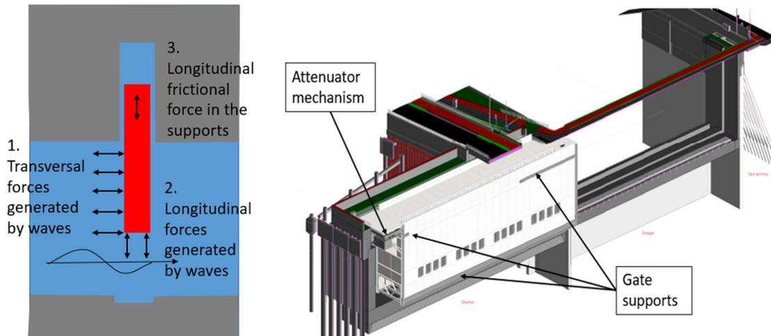
Figure 1: Overview of wave forces on the gate
