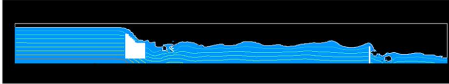
Figure 2: Snapshot of CS1 ( $h_{front}=0.45m$ ,  $h_{weir}=0.2m$ )
