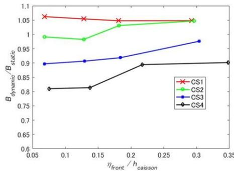
Figure 3: Ratio of dynamic and static buoyancy ( $h_{weir}=0.2m$ )
