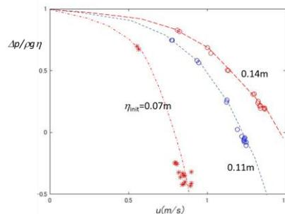
**Figure 1: Relationship between velocity and pressure decrease at the top of the caisson**
