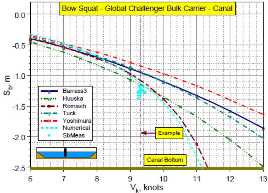
Figure D-13: Bow squat for Global Challenger Bulk Carrier, Panama Canal,  $L_{pp} = 216$  m,  $B = 32.2$  m,  $T = 11.7$  m,  $C_B = 0.83$ ,  $h = 14.2$  m ( $h/T = 1.21$ ),  $W = 152.4$  m,  $W_{Top} = 206.4$  m and  $n = 1.9$
