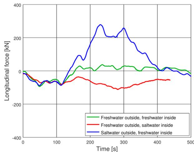
**Figure 2: Impact of density driven flow on the longitudinal ship forces for the “horizontal breaker bars” configuration**
