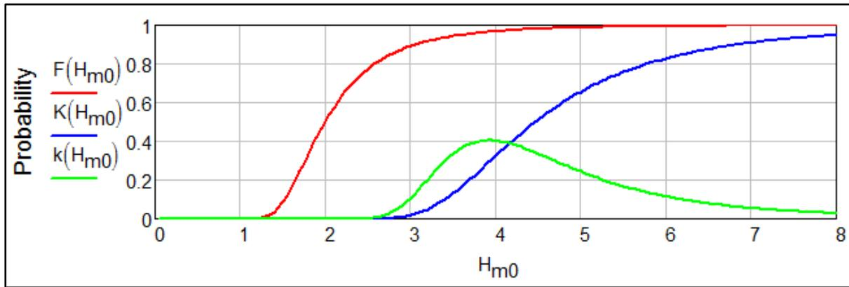
**Figure 12 Probability functions for the south breakwater (similar for the north breakwater)**
