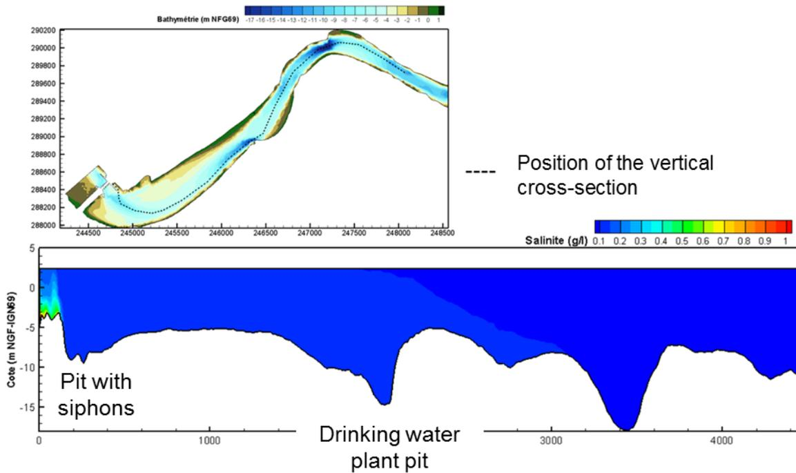
Figure 10: salt intrusion cartography – new lock without siphon
