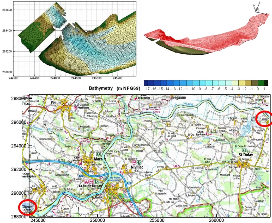
Figure 4: extend and mesh of the numerical model
