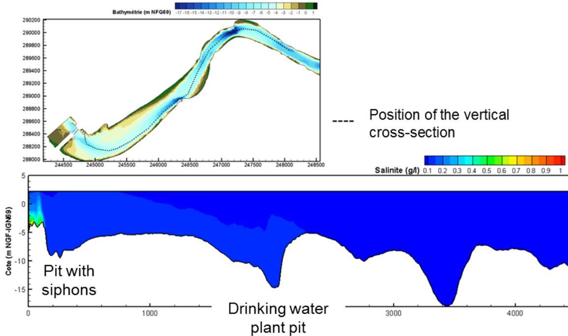
**Figure 8: salt intrusion cartography – new lock with siphons**
