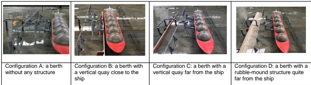
**Figure 3. Views of the different studied configurations**
