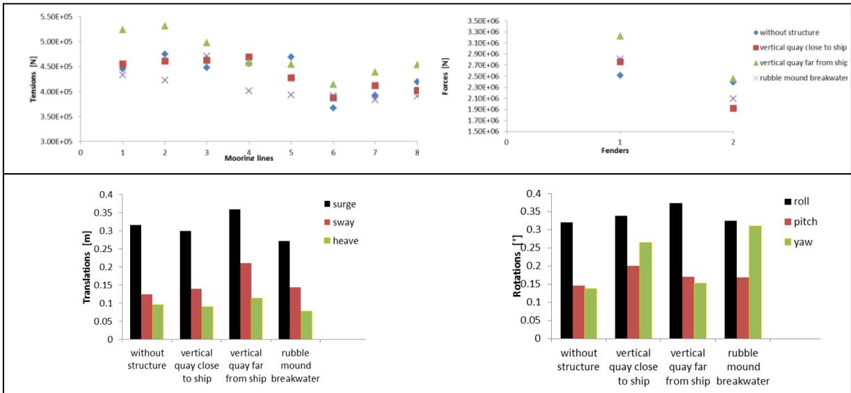
Figure 11.: Influence of harbour structures - quartering seas -  $H_{m0} = 1\text{ m}$  –  $T_p = 10\text{ s}$  - 18m water depth
