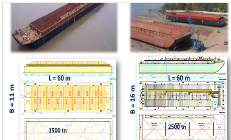
**Figure 3 – Dimensions of “Mississippi” and “Jumbo” barges**
