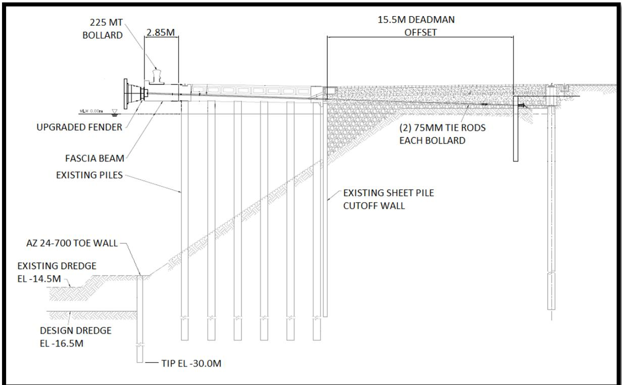
Figure 4: Berth 8 Typical Section after Upgrades
