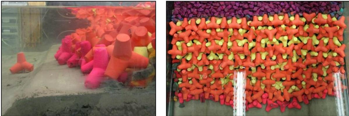
**Figure 6 – Displaced toe and slumping of breakwater armor.**
