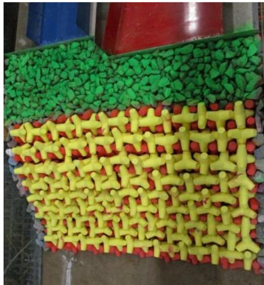
**Figure 8. Top – deep water cross-section design; bottom - constructed deep water cross-section breakwater.**
