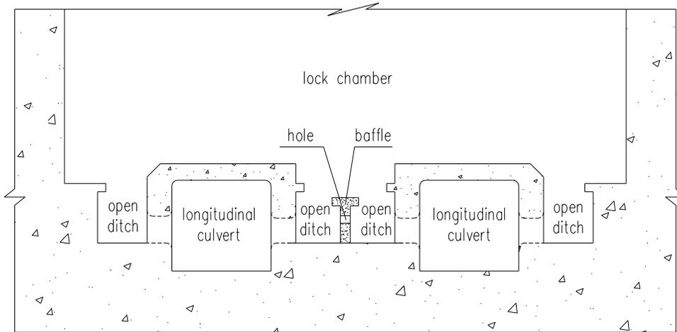
**Figure 6: Cross section of lock chamber after improvement**
