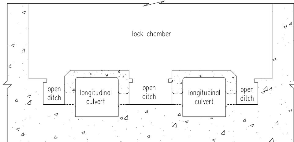
Figure 2: Cross section of lock chamber for Xijin 2<sup>nd</sup> lane lock
