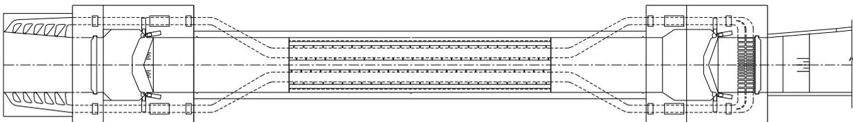
Figure 1: Initial layout of In-chamber Longitudinal Culvert System for Xijin 2<sup>nd</sup> lane lock
