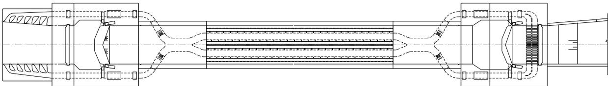
**Figure 7: Layout of improved In-chamber Longitudinal Culvert System for Xijin 2<sup>nd</sup> lane lock**
