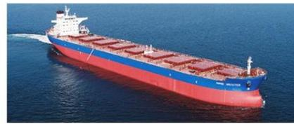
A. Bulk Carrier in Ballast Condition
