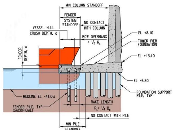
Figure 18: Ship Bow Crushing and Bridge Pier Geometry
