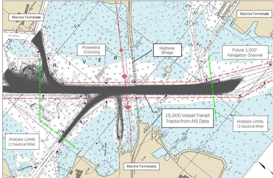
Figure 9: AIS Vessel Tracks at Bridge Location
