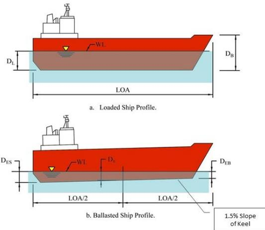
**Figure 8: Ballasted Vessels**
