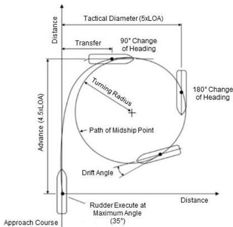
Figure 13: Aberrant Ship Turning Circles
