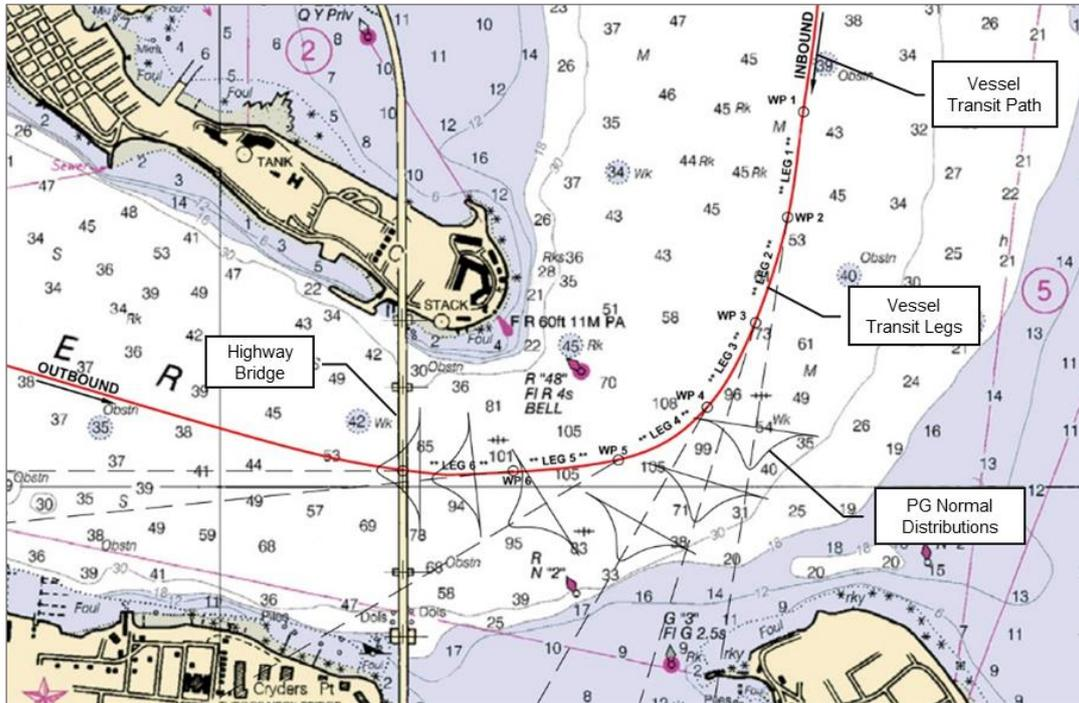
Figure 16: Illustration of Curved Channel Approach to Bridge
