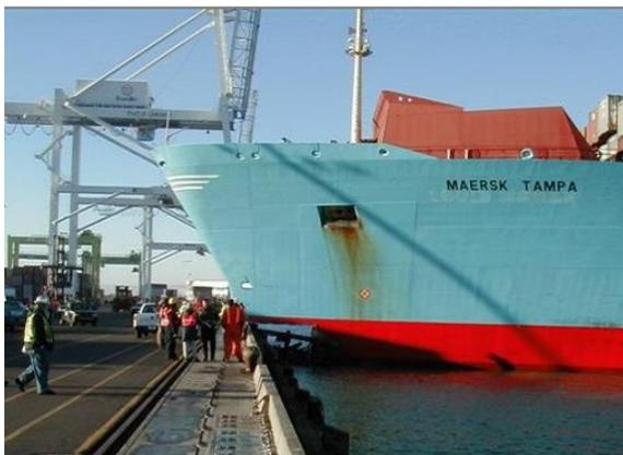
Figure 17: Ship Bow Crushing
