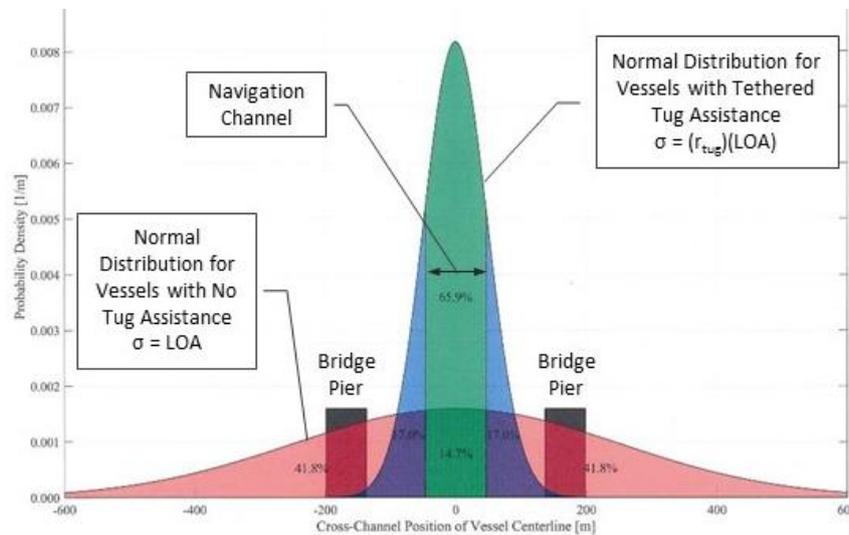
Figure 11: Tethered Tug Adjustment Factor
