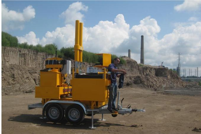
Figure 6. Cone Penetration Test
