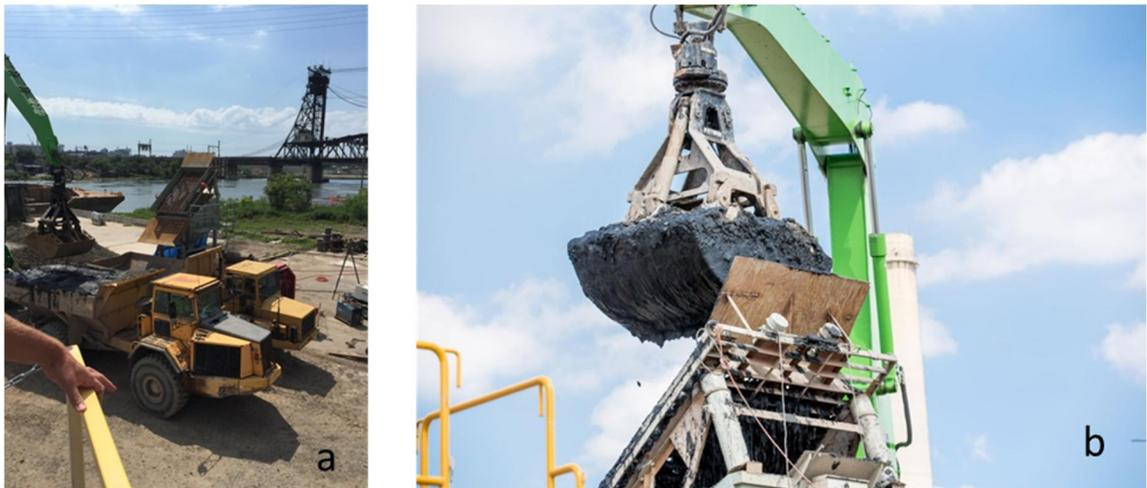
Figure 1. (a) Vibrating with being loaded from a truck (b) Screen and vibrator configuration.
