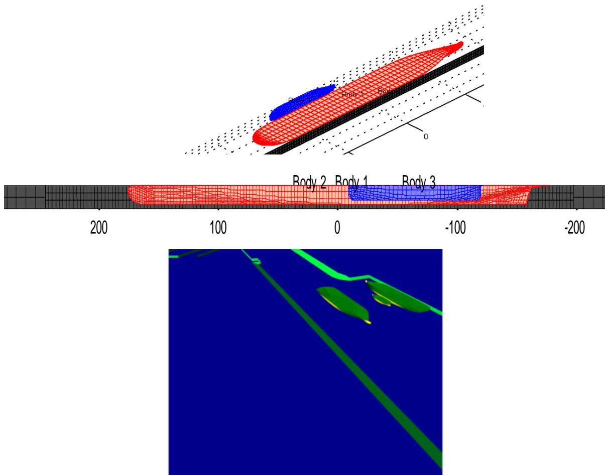
**Figure 4: mesh files for motion/mooring analysis (top) and passing vessel analysis (bottom)**
