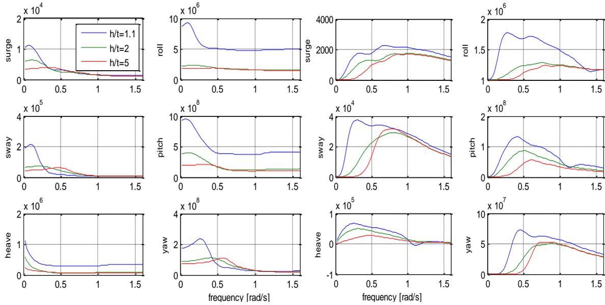
Figure 1: Effect of UKC on added mass and potential damping (mt, kNms)
