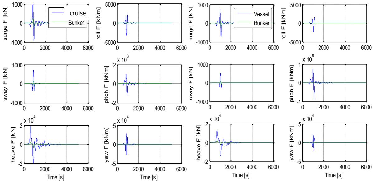
Figure 5: passing vessel forces (7kn right, 6kn left)
