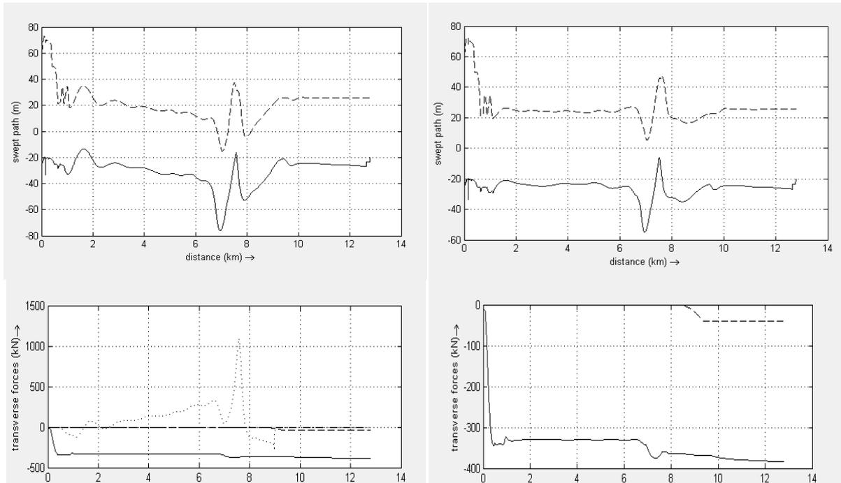
Figure 10: Effect of bank suction on swept path
