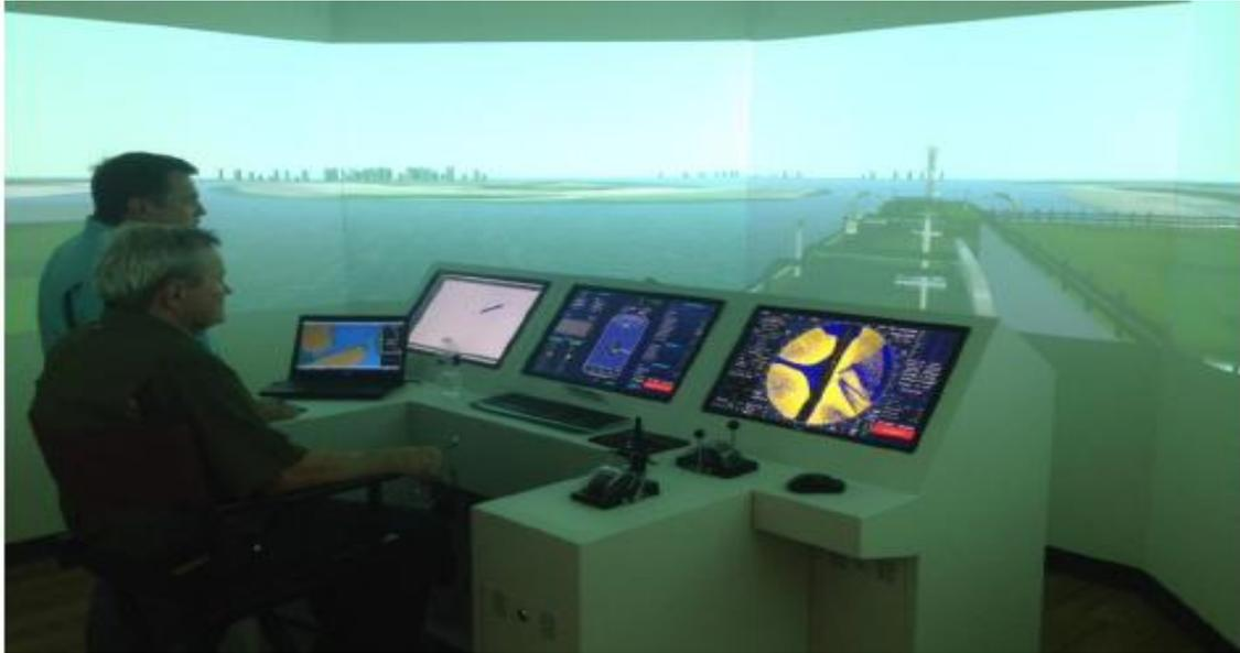
Figure 7: MARIN Houston real-time bridge simulator
