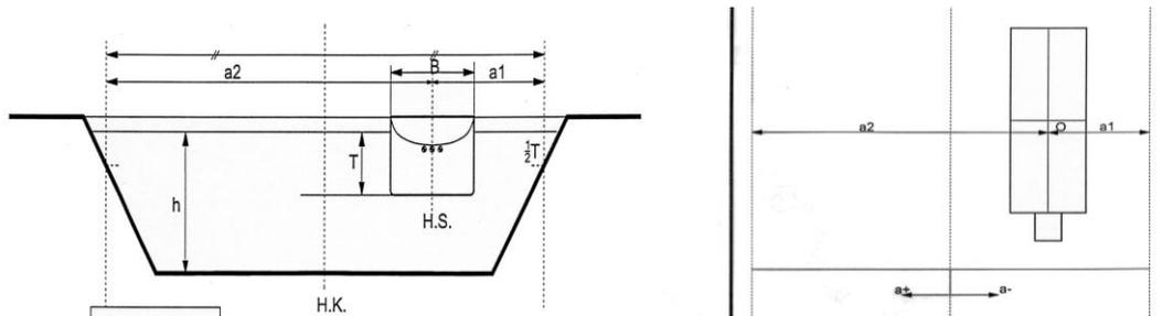
Figure 9: Dimensions used in the Norrbin bank suction model
