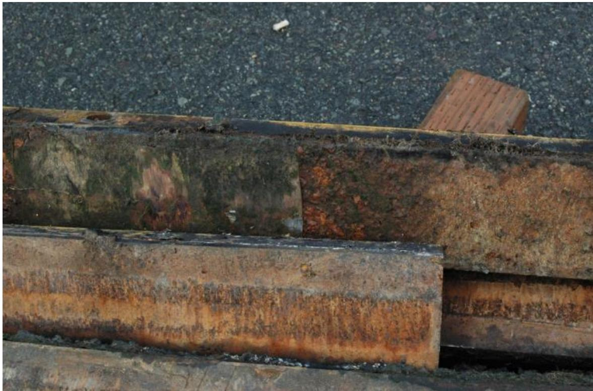
**Figure 1: Corroded and Abraded Carbon Steel Miter Blocks**
