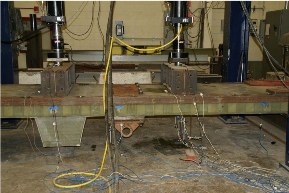
**Figure 6: Flexure Test of Prototype FRP Wicket Gate**
