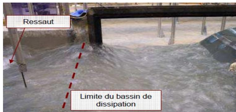
Figure 17 Hydraulic jump after the limit of basin
