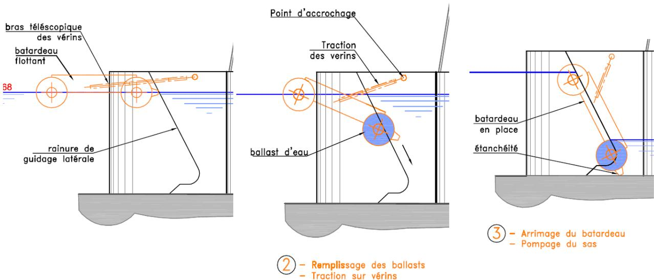
figure 24 - Le Coudray : 3 phases to put the bulkhead in final place
