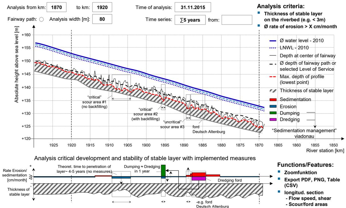
Figure 13: Assessment of critical scour areas based on thickness of stable layer, sedimentation and erosion rates with systematic dredging in sedimentation areas and dumping in scour areas
