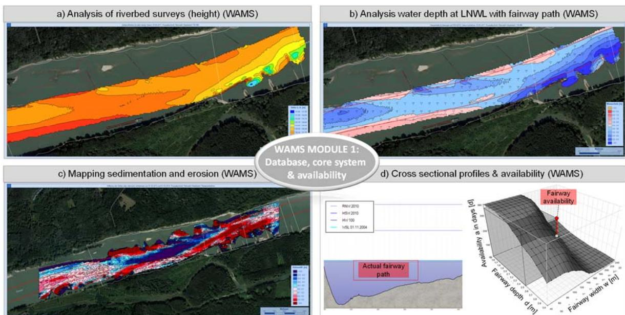
Figure 5: WAMS Module 1 with automatic analysis of a) Riverbed survey, b) Water depth, c) Sedimentation & erosion, d) Cross sectional profiles & availability calculation
