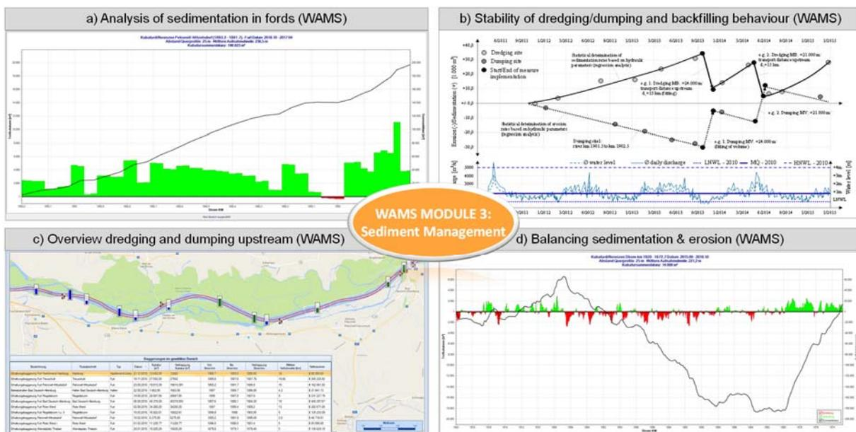
Figure 8: WAMS Module 3 with a) Sedimentation in fords, b) Stability of dredging/backfilling, c) Overview conducted dredging and dumping, d) Balancing sedimentation and erosion
