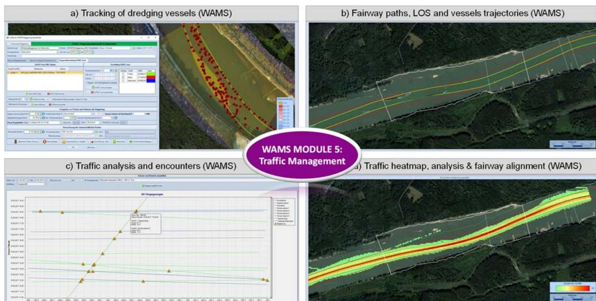
Figure 11: WAMS Module 5 with a) Tracking of dredging measures, b) Fairway paths and levels of service, c) Traffic analysis and encounters, d) Traffic heatmap, analysis & fairway alignment
