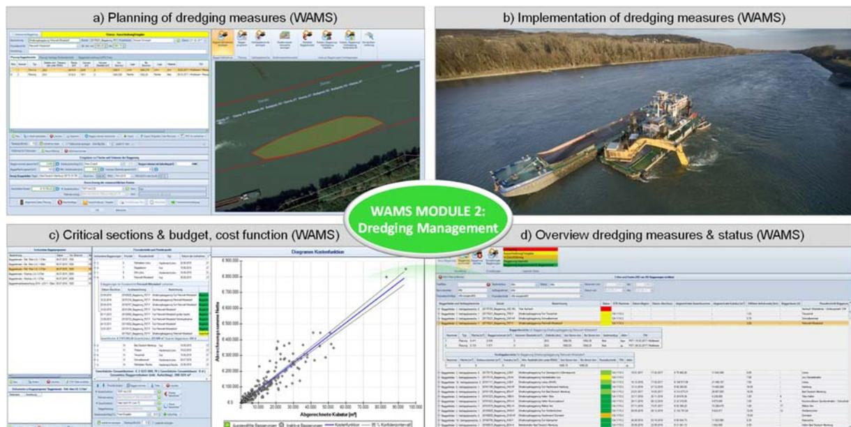
**Figure 7: WAMS Module 2 with a) Planning of dredging, b) Implementation & controlling, c) Critical sections, costs and budgeting, d) Overview status and implementation of dredging**
