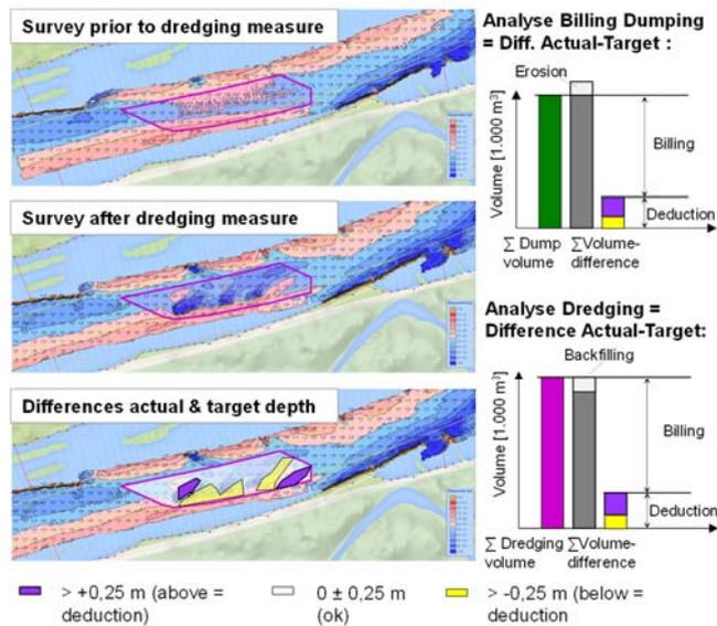
**Figure 6: Calculation of dredging and dumping volumes controlling for deviations due to backfilling and differences to target depth**
