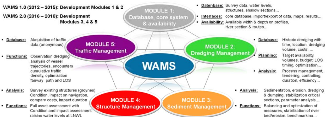
**Figure 4: Overview developed modern modular Waterway Asset Management System WAMS of viadonau being operational since 2015**
