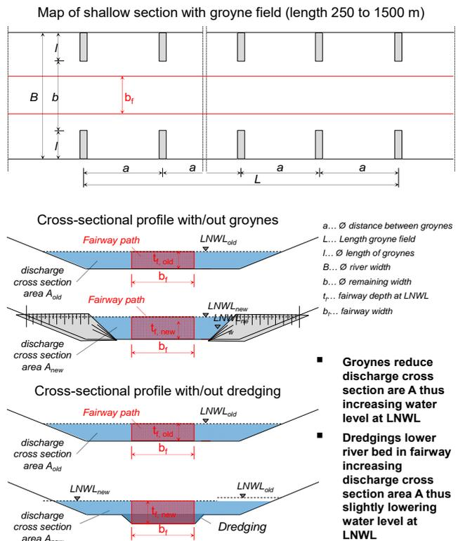
**Figure 9: Impact of river engineering measures and dredging in the fairway path on available depth at low navigational water levels (LNWL)**
