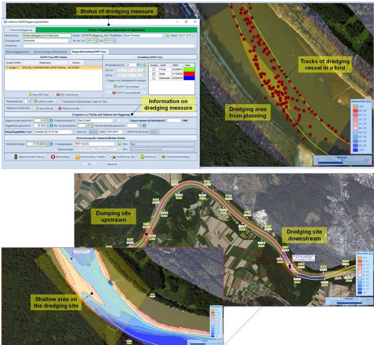
Figure 12: Automated analysis of dredging measure status with monitoring of dredging vessels and results based on transponder data and multi-beam surveys (WAMS)
