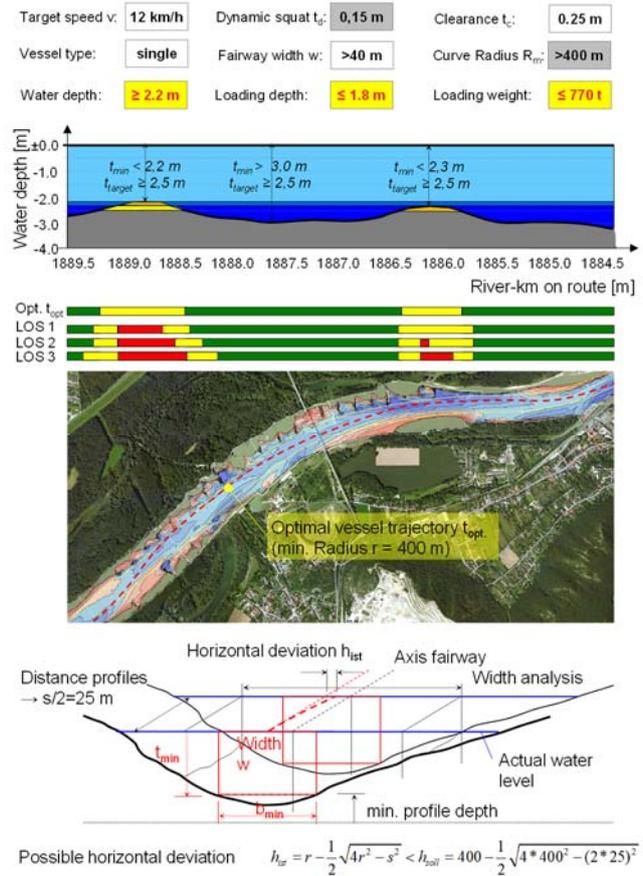
Figure 13: Example for a simplified route planner with calculation of trajectory with max. water depth and possible loading of a vessel
