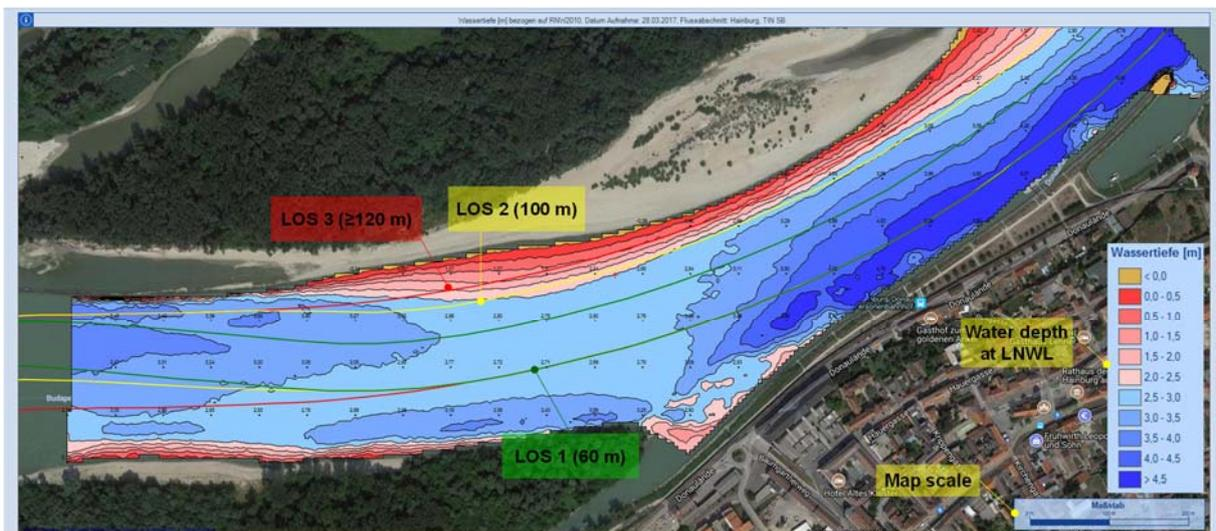
**Figure 9: Automated analysis of water depths (LNWL 2010) based on multi-beam survey and water levels with fairway alignment and LOS 1, 2, 3 in 2017 (WAMS)**
