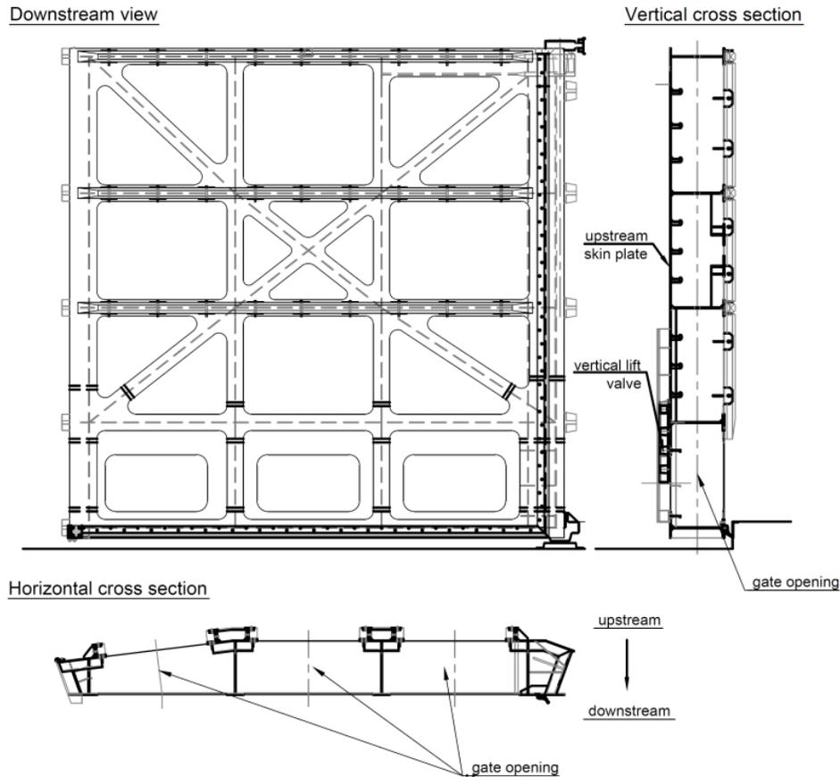
**Figure 2: Mitre gate leaf with three leveling openings**
