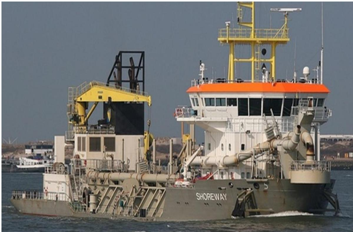
Figure 3: The dredging of the main channel for Bahia Blanca's 97 kilometer estuary was done by the TSHD "Shoreway" from Royal Boskalis Westminster n.v. (hopper capacity 5,600 m<sup>3</sup>).
