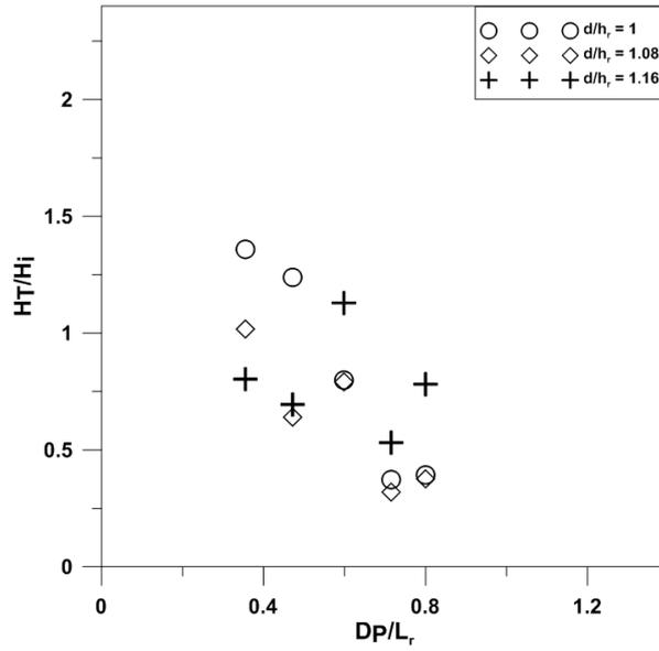
Figure 8: Wave Transformation for  $L_r/L = 0.88$  to  $0.93$  &  $H/d = 0.086$  to  $0.1$
