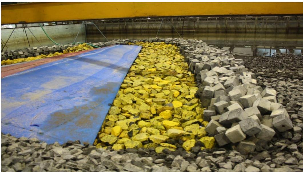
Figure 3: Armour stones and concrete cubes with holes
