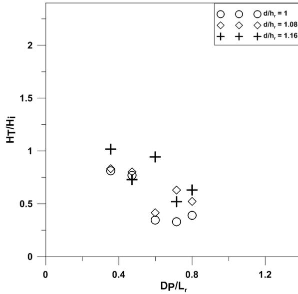
Figure 10: Wave Transformation for  $L_r/L = 0.88$  to  $0.93$  &  $H/d = 0.25$  to  $0.3$
