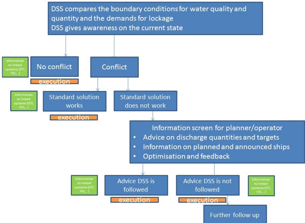
**Figure 7 : schematic representation of DDS flow chart**
