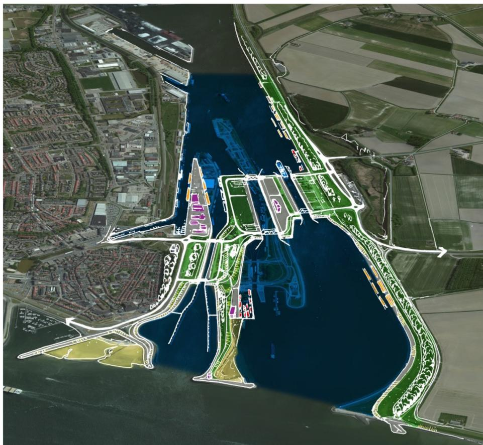
**Figure 6 : sketch of the lock complex at Terneuzen. The New Lock will be constructed centrally in the complex and will replace the original Middensluis (VNSC, 2015)**
