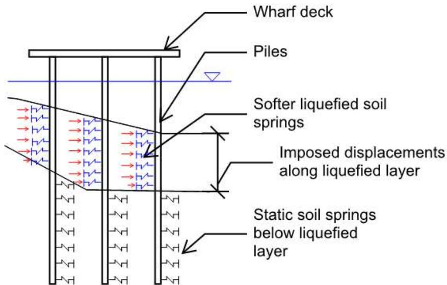
**Figure 5: Kinematic Displacement Applied at Softened Soil Spring**
