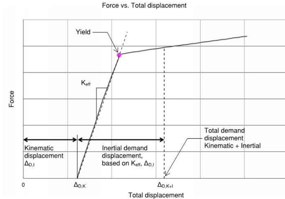
**Figure 3: Pushover Curve for Kinematic plus Inertial Analysis**
