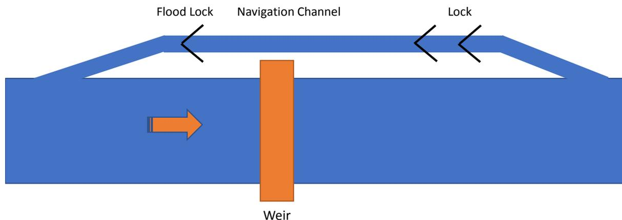
The owners, managers and operators of inland navigations all know the difference in levels and have a historical record of the variation of flow over time at the at each weir and lock location. Whilst the water has other uses, particularly for navigation and compensation flows, any surplus can be put to good use generating power.
