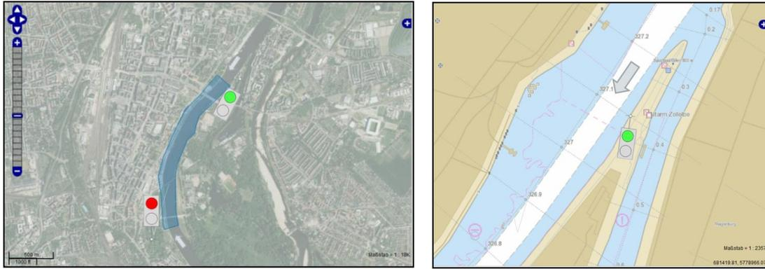
Figure 5: Current switching status of signals, visualized in Inland ECDIS
