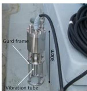
Figure 9: Instrument for In-situ Bulk Density Measurement
