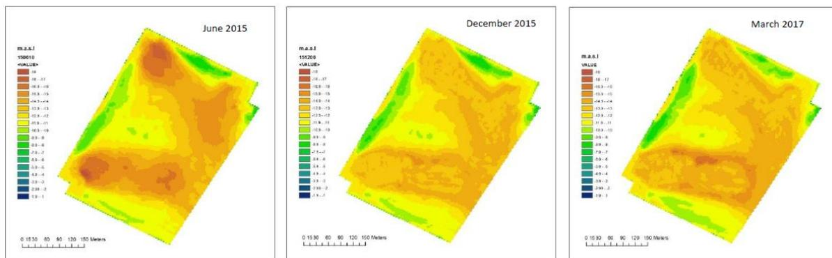
Figure 1: Evolution of the bathymetry along the harbour
