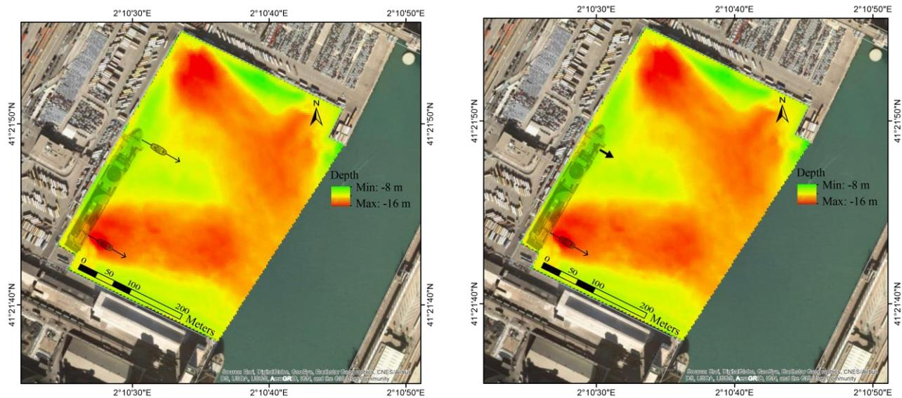
**Figure 16: Representation of alternative unberthing manoeuvres with tugs**
