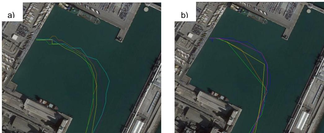
**Figure 7: West quay undocking manoeuvres scenario (a) Calm weather (08/06/16-blue, 17/06/16-orange, 20/06/16-purple, 01/07/16-yellow and 06/07/16-green) (b) Bad weather (13/01/17-blue, 15/01/17-orange, 18/01/17-purple, 20/01/17-yellow and 23/01/17-green)**
