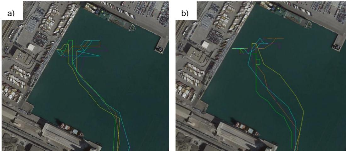
**Figure 4: West quay docking manoeuvres scenario (a) Calm weather (8<sup>th</sup> June (blue), 17<sup>th</sup> June 2016 (orange), 19<sup>th</sup> June 2016 (purple), 1<sup>st</sup> July 2016 (yellow) and 6<sup>th</sup> July 2016 (green)). (b) Heavy weather (12<sup>th</sup> January 2017 (blue), 14<sup>th</sup> January 2017 (orange), 17<sup>th</sup> January 2017 (purple), 20<sup>th</sup> January 2017 (yellow) and 23<sup>th</sup> January 2017 (green))**
