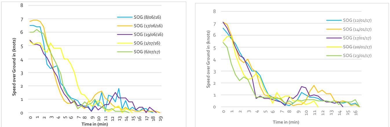
**Figure 6: Speed over Ground (SOG) for entrance manoeuvrings considered in calm (left) and bad (right) weather**
