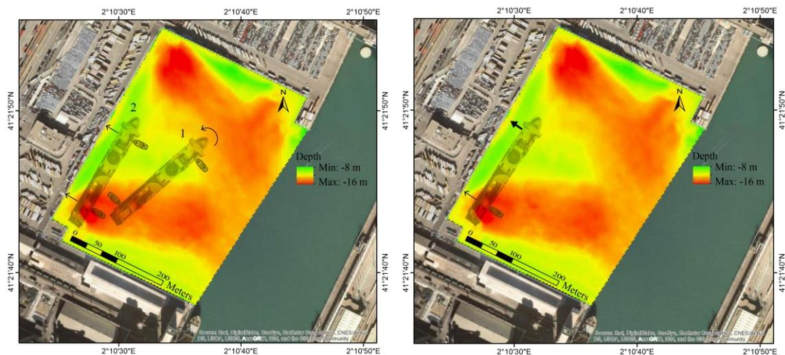
**Figure 15: Representation of alternative berthing manoeuvres with tugs**
