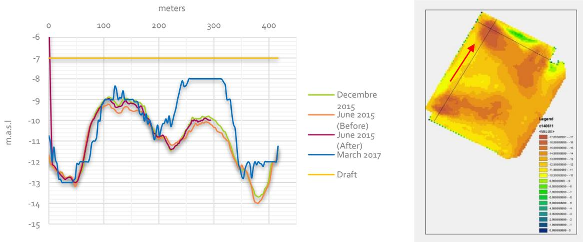
Figure 12: Evolution of the bathymetry along a section parallel to the west quay, from south to north
