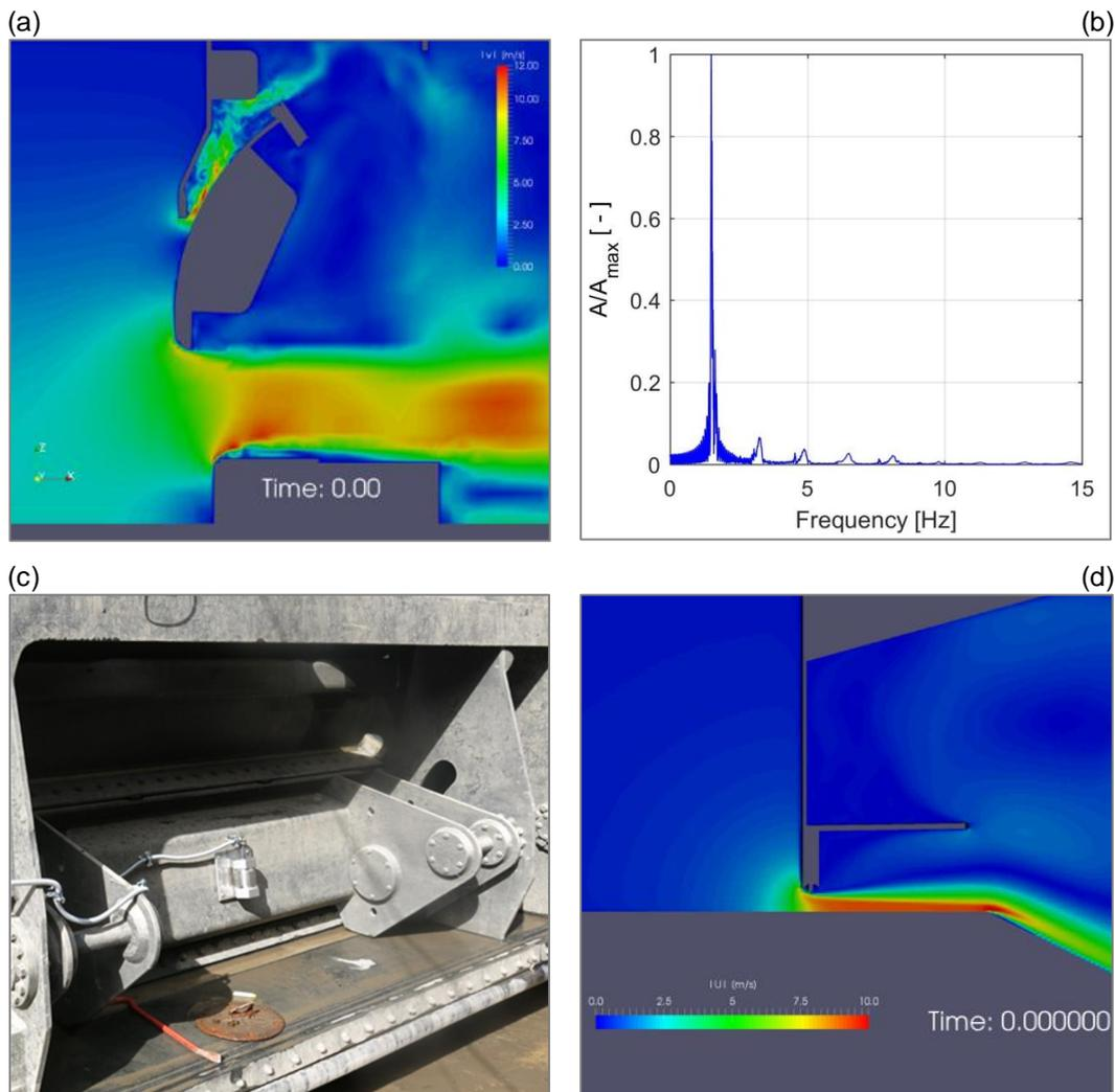
**Figure 2: Applied methods: (a) numerical simulation of a filling valve; (b) Frequency analysis of a measuring signal; (c) acceleration sensor at filling valve of a mitre gate and (d) numerical simulation of fluid-structure interaction of a lifting gate**
