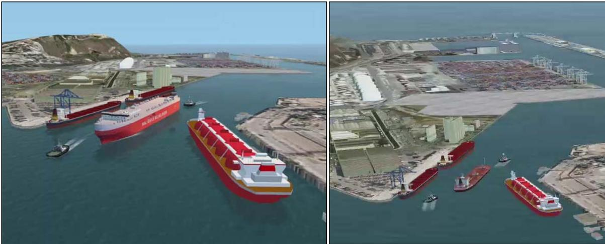
**Figure 15: Real-time simulator manoeuvres: approach manoeuvre of the car carrier and departure manoeuvre of the tanker**
