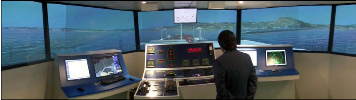
**Figure 14: Siport21 real-time simulator in operation**
