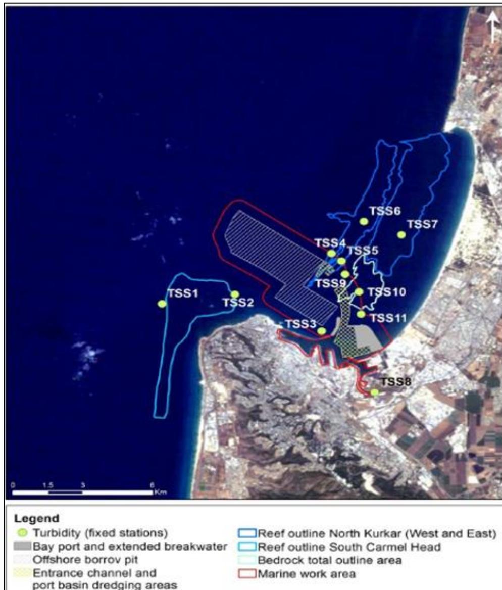
Figure 8: 11 turbidity sensors for on-line monitoring dredging
