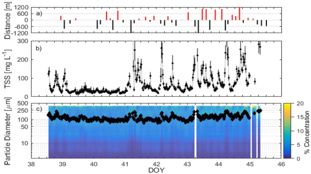
**Figure 5: a) Location of Dredge Placements Relative to Frame (b) LISST TSS Concentration Time-Series (c) LISST Particle Size Distribution and  $d_{50}$  Estimates**
