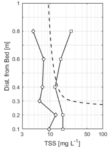
**Figure 6: BBL Suction Profiler and Rouse Concentration Profile**
