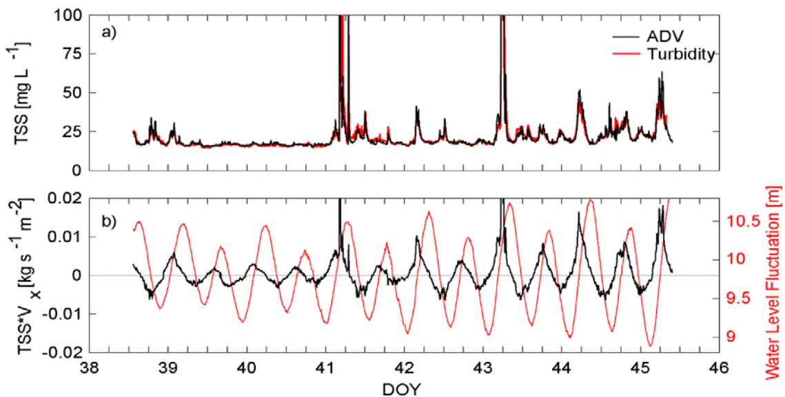
**Figure 4: a) Calibrated TSS Concentration Time-Series b) Horizontal Concentration Flux Along the Principle Flood/Ebb Axis**
