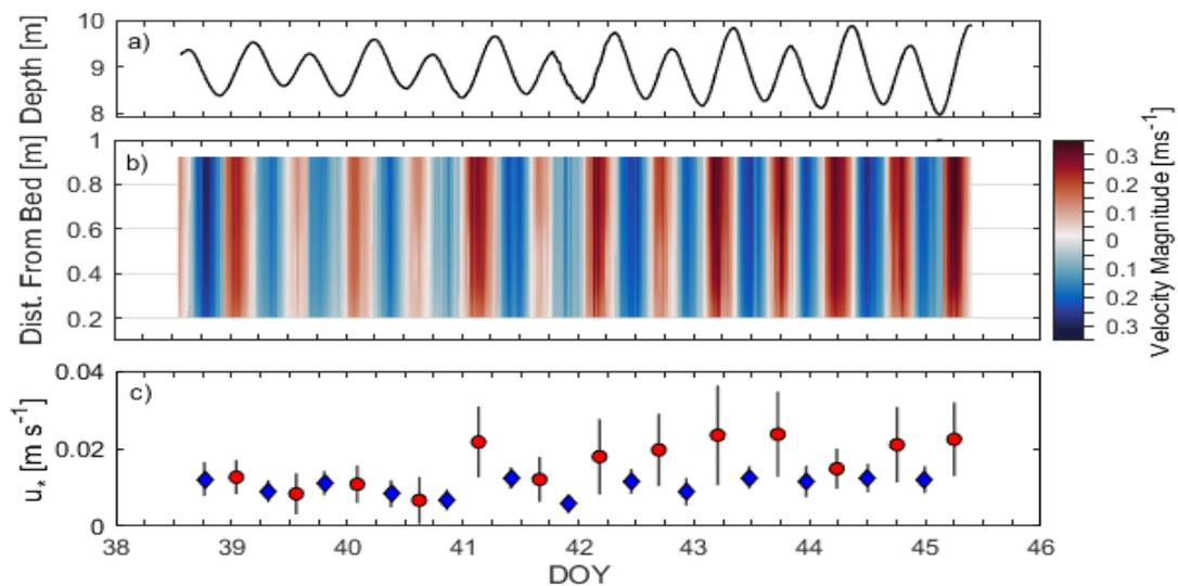
**Figure 3: (a) Water Level Fluctuations (b) Near-Bed Horizontal Velocity Magnitude (North-East) and (c) Friction Velocity Estimates**
