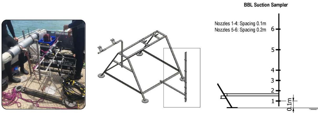
Figure 2: Deployment Frame and BBL Suction Profiler
