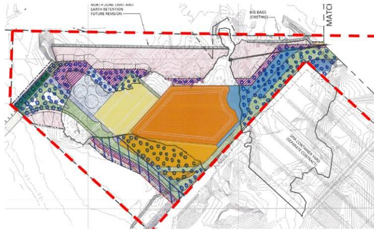
**Figure 3: Cut and fill areas at project start date (access road is not shown)**
