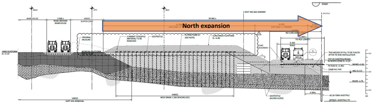
Figure 10: Cross section north yard with typical surcharge (here 1.5m high for 2t/m<sup>2</sup>)
