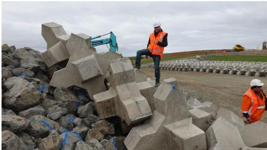
Figure 5 - Xbloc placed on a test slope
