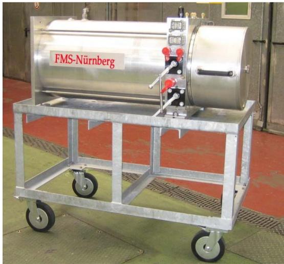
**Fig. 11: Typical Hydraulic Compact Unit**
