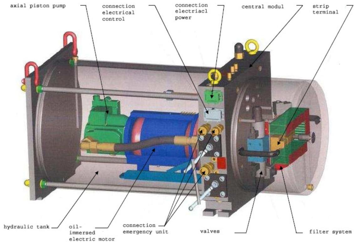
Fig. 10: Hydraulic Compact Drive unit - general arrangement
