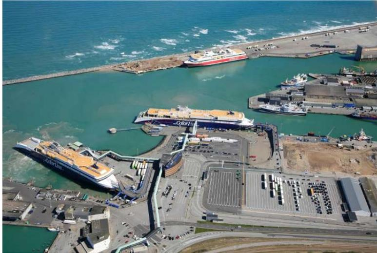
**Figure 10: The ferry berths in the center of the port area and new combined ferry and container berth along the north breakwater**
