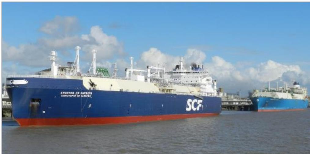
**Figure 25: Trans-shipment at Montoir de Bretagne between an Ice-breaking LNG Carrier and a conventional LNG Carrier**
