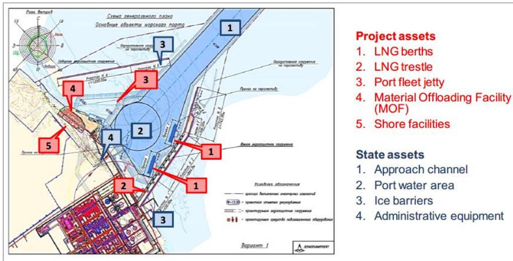
Figure 9: The general lay-out of the Arctic Port
