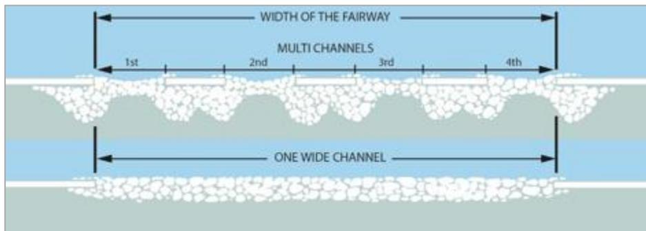
**Figure 6: Multi-channels approach for the North Access channel to Sabetta**
