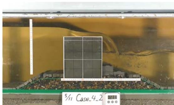
(b) Test against Tsunami in wave flume
