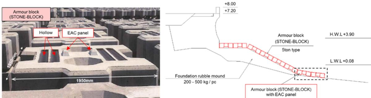
Figure 19 : Armour blocks attached with EAC panels and Cross-section
