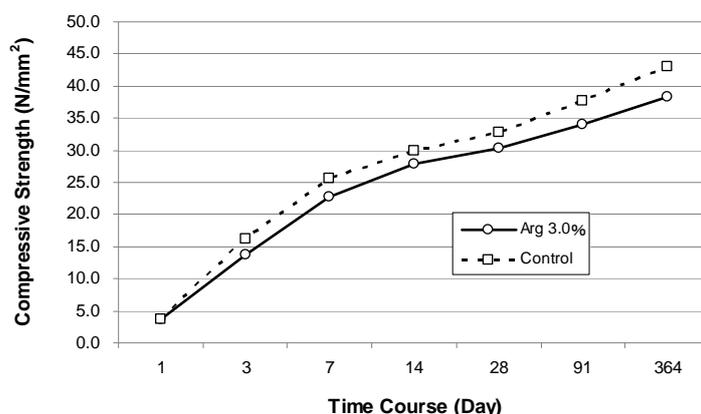
Figure 10 : Temporal Change of Compressive Strength
