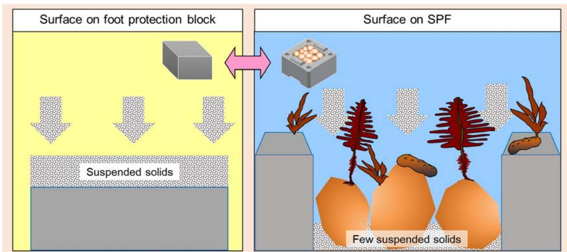
Figure 9 : Diference between foot protection block and SPF
