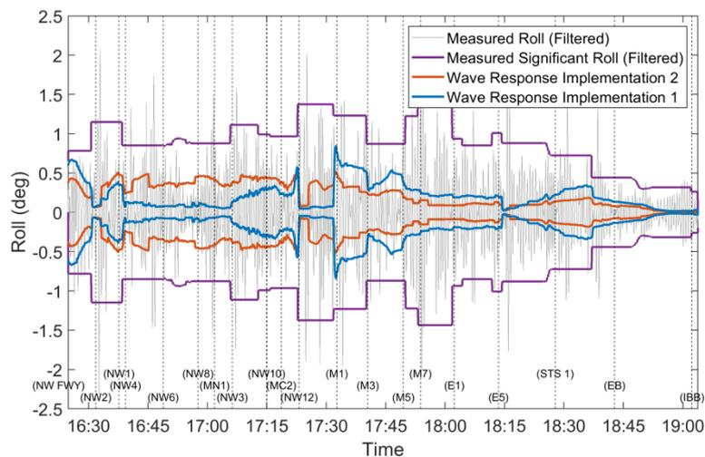
**Figure 8: C1 Filtered Roll Validation (Container Vessel, Inbound)**
