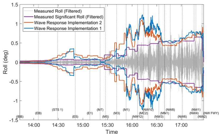
Figure 7: B3 Filtered Roll Validation (Bulk Carrier, Outbound)
