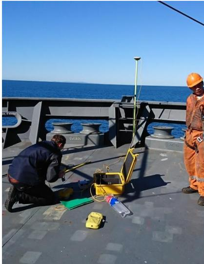
Figure 1: DGPS Setup on Bow
