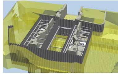
**Figure 15 - Phasing – Closure period 2 – Unification of small cofferdams**
