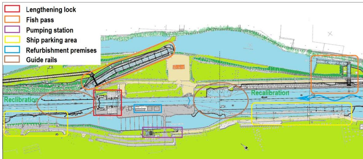
**Figure 4: Plan view of the lock site**
