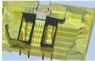
**Figure 12 - Phasing – Closure period 1 – Smalls cofferdams and piles**
