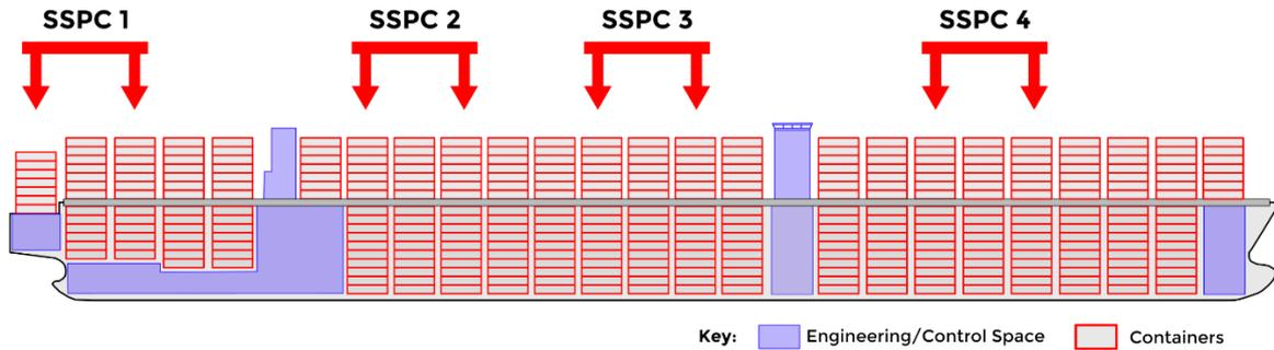
Figure 11: Typical ULVC showing possible SSPC locations
