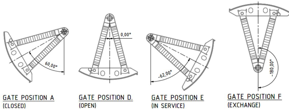
**Figure 6: Gate positions (excl. position -120°, in service)**
