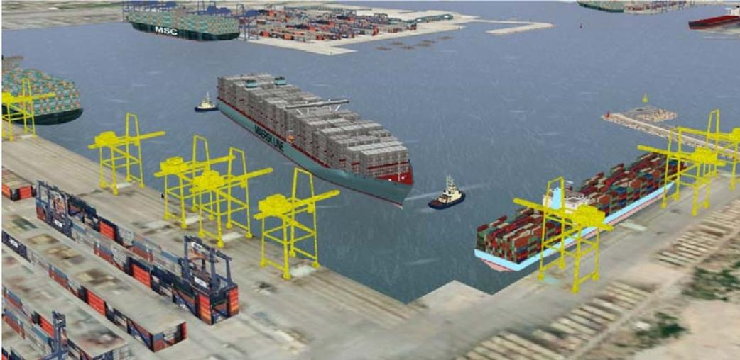
**Figure 11: 3E Maersk containership access manoeuvre. Simulator image**
