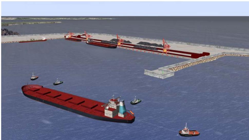
Figure 9: Verification of fairway and basin for Valemax bulkcarrier. Simulator image
