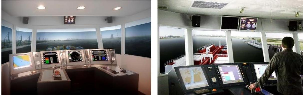
Figure 6 Full mission bridge simulators 225 and 360+ at FHR
